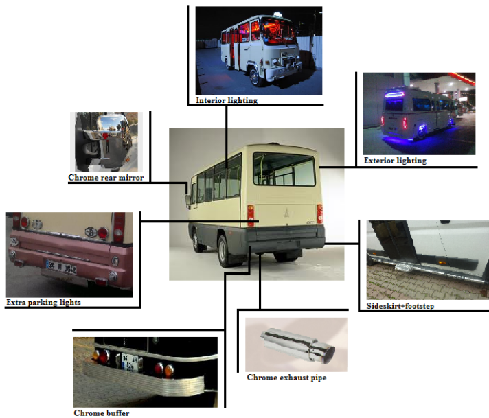
Figure 3 - Some elements of exterior modifications in dolmuşes from back view (Prepared by Elçin Tezel).*
