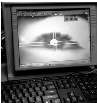
Figure 2 - Deformations in the CR can be used to calculate point-of-gaze across an image.
